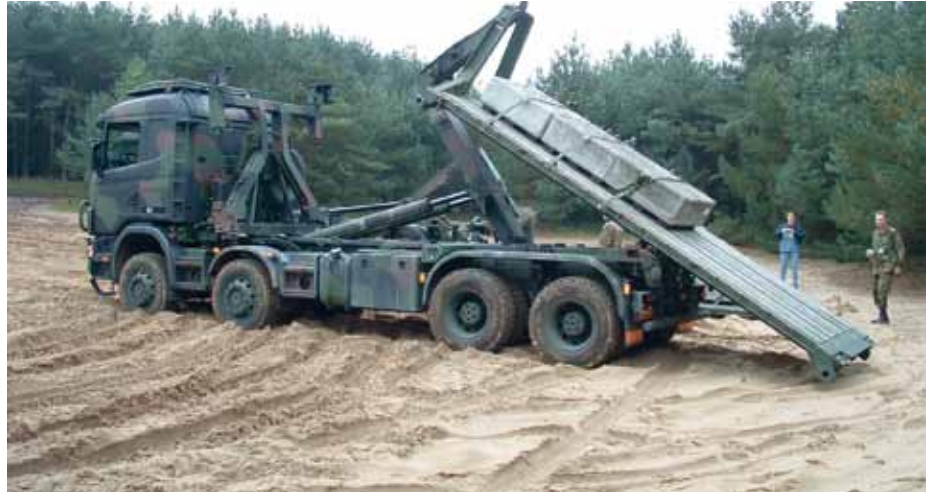
Multilift MSH165 Military Load Handling System handling Scania Flatrack
