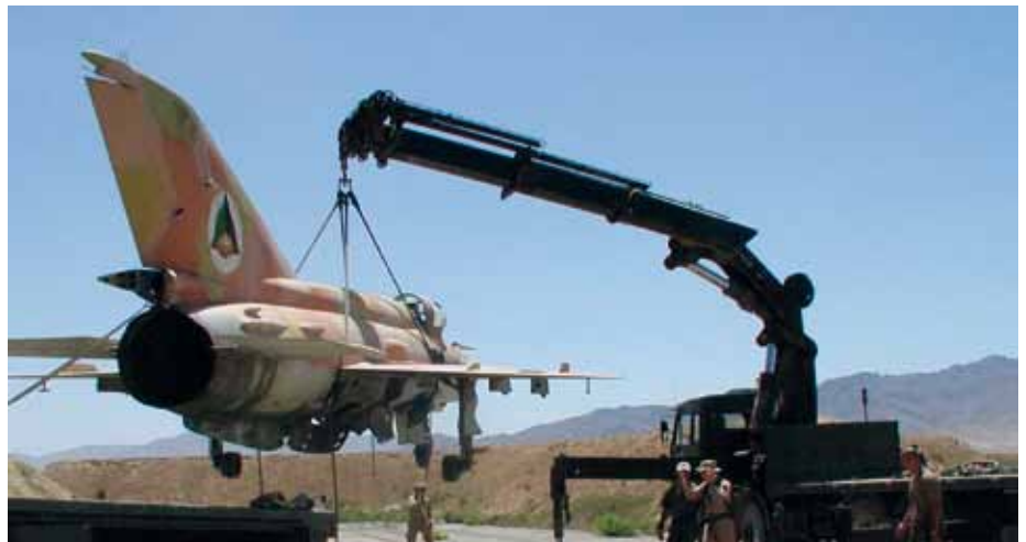
Hiab lorry loader crane in use by a Military end user for airfield clearance
