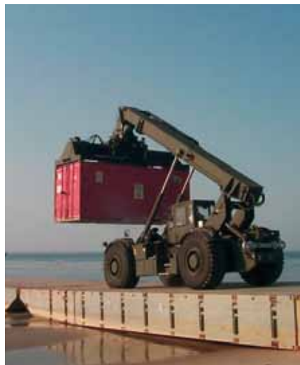
KALMAR RT240 RTCH unloading vessels via pontoons
