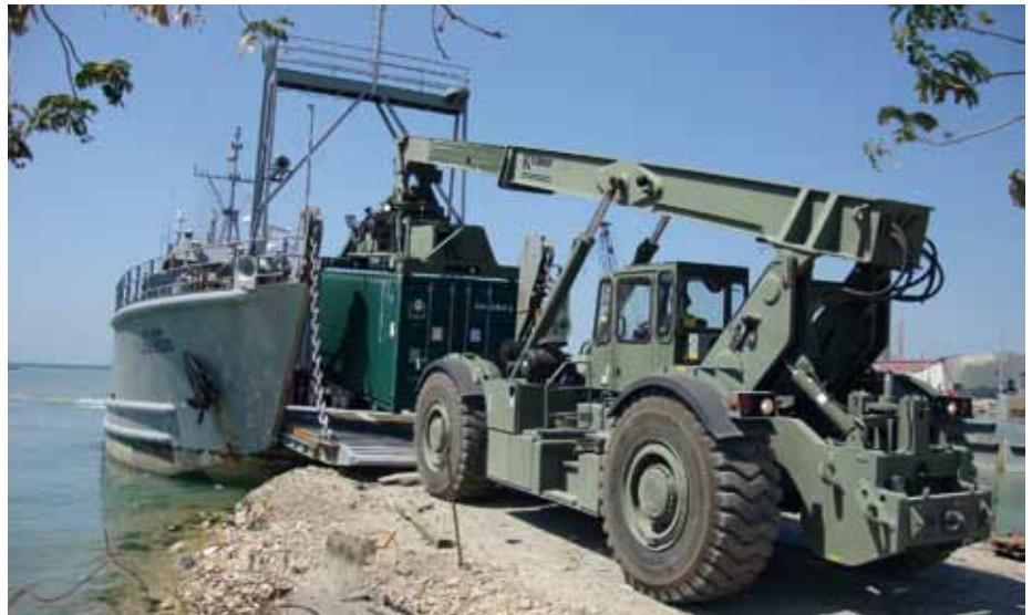
KALMAR RT240 RTCH unloading landing vessel
