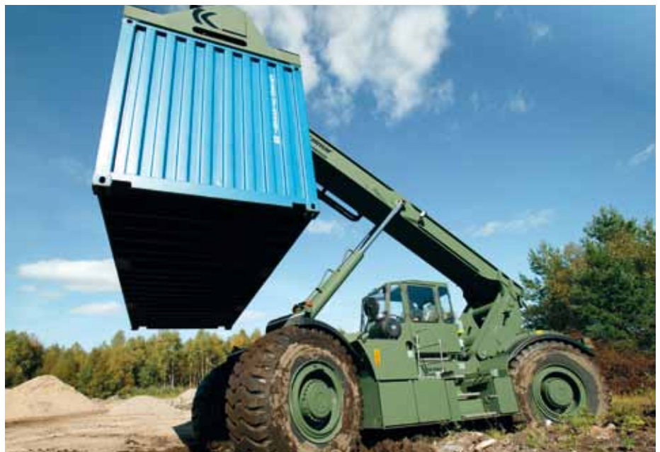
KALMAR RT240 Rough Terrain Container Handler handling a 20' ISO container
