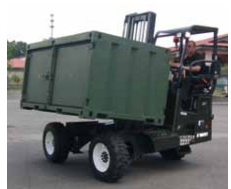
MOFFETT M8 - 4 Way in "Cat C" compliant version drives in forward, rearward, left and right direction
