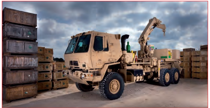
HIAB 2222 ATF-1 crane on medium FMTV wrecker vehicle US Army
